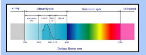
UV-C rays are harmful to human skin and eyes as they have a wavelength of 200-280 nm. Avoid direct contact with the UV-C lamps inside the device.
